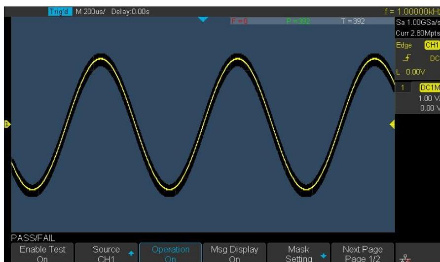
Figure 88 Pass/Fail Test
