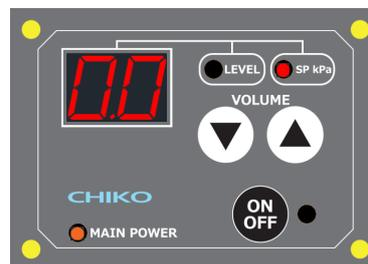
3. Press [ON/OFF] on the operation panel to start operation of the device. (The operation lamp will light up.)
