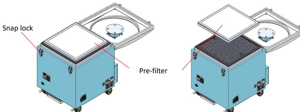
2. Remove the activated carbon cassette by pulling the handle.
