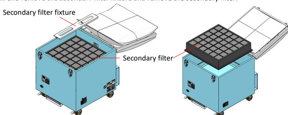
3. Install the new primary filter and attach the secondary filter fixture by pushing it in.
