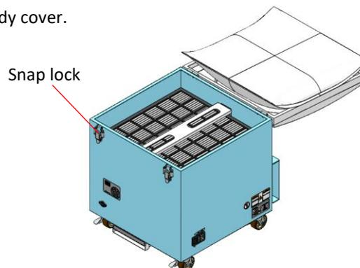
2. Pull and remove the secondary filter fixture and remove the secondary filter.
