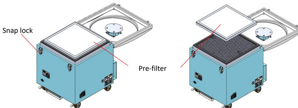
3. Remove the filter retainer.
